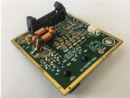
Figure 17. bPOL48V using the FEASTMP inductor.
