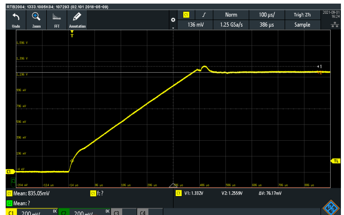
Figure 8: Output voltage measured on a sample of bPOL2V5_V3.3 at room temperature during the Soft Start, for V_{in}=2.5V , V_{out}=1.2V , I_{out}=0A . The small overshoot on V_{out} at the end of the Soft Start is inherent to the operation of the controller.
