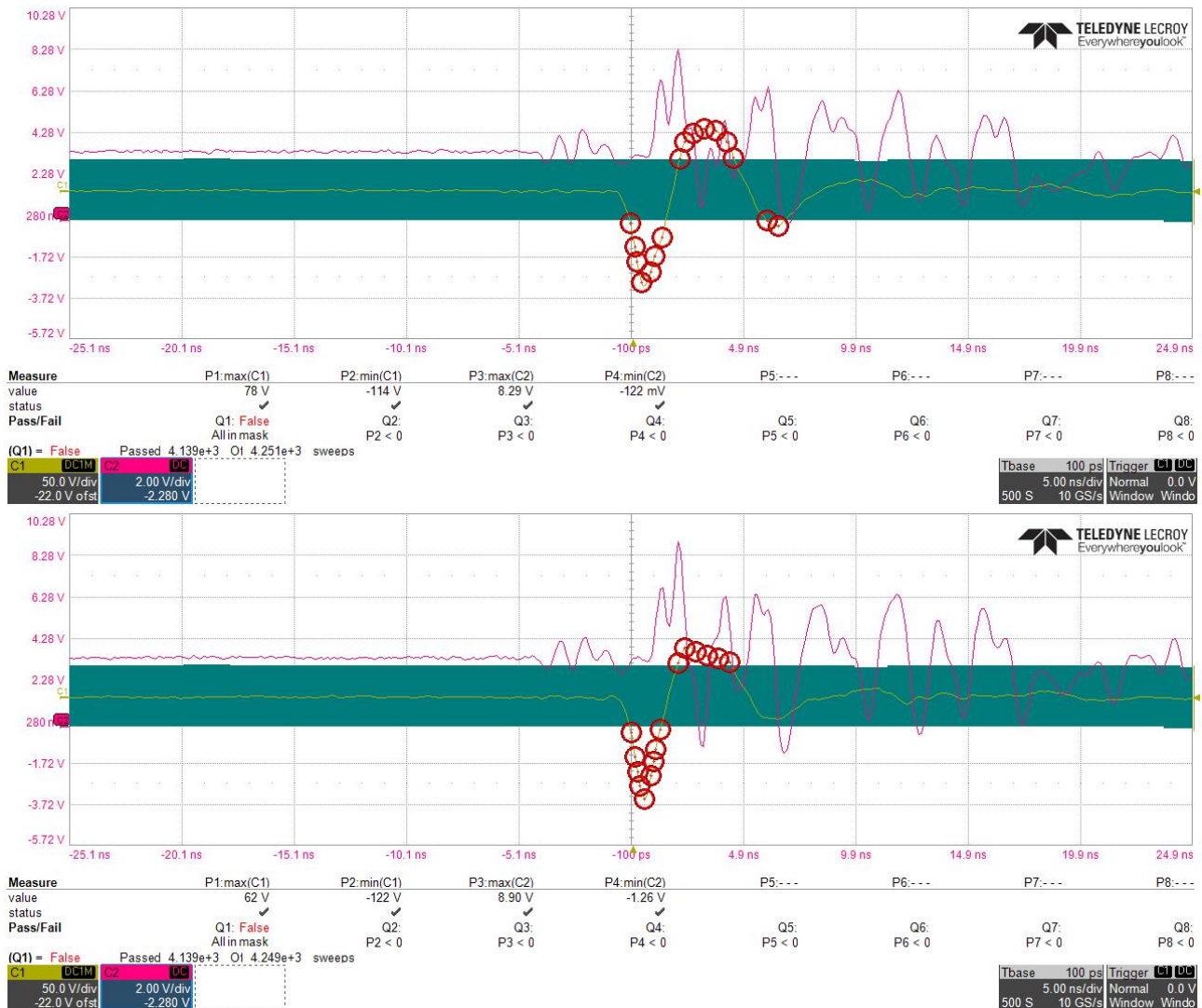
Figure 4: Screenshots of the oscilloscope used to observe the Enable and V33Dr nodes during ESD discharge tests. The yellow trace (with red dots) is the enable, the purple is V33Dr. The negative peak of the enable is 114V in the top and 122 V in the bottom image. V33Dr can raise to almost 9V (bottom image), making a damage on that node plausible.
