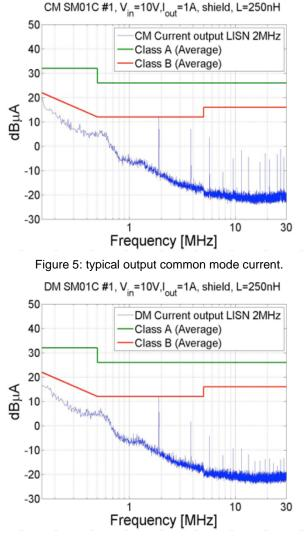
Figure 6: typical output differential mode current.
