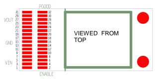
Figure 2: Top view and pin numbering of the power interface
