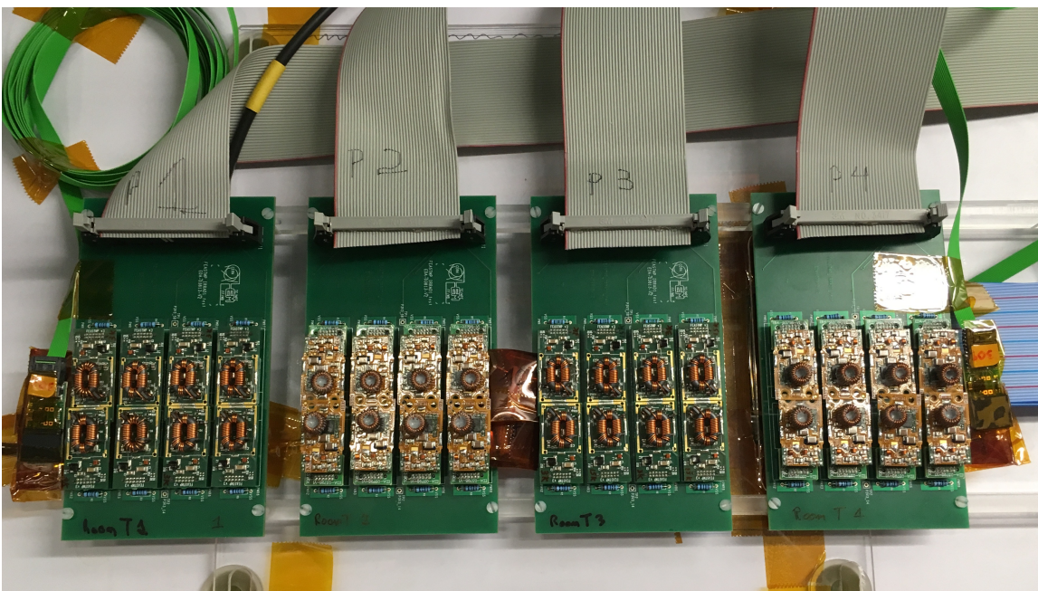
Figure 13: The 4 motherboards installed in the outer side of the box cover, ready for the installation in the experimental area. The dosimeters are visible. All boards had the standard sequence of I-V sweep and disable-enable, but the last board to the right was powered by a separate supply steadily at 8V (not controlled by the PC).
