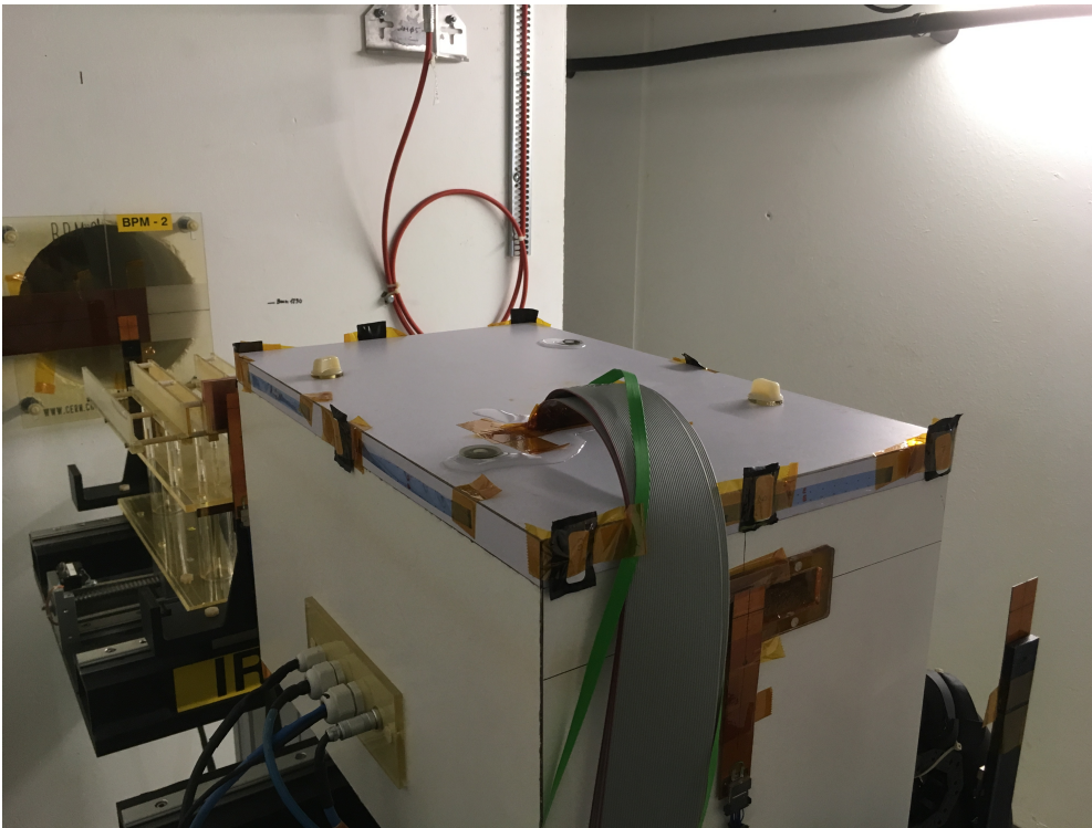
Figure 5: The closed cold box in its location inside the IRRAD experimental area. The Cu target is visible, as well as the 4 grey flat cables for the acquisition system and bias. The green cables are used for active dosimeters inside the box. Passive dosimeters were installed all around the box, on the cover.
