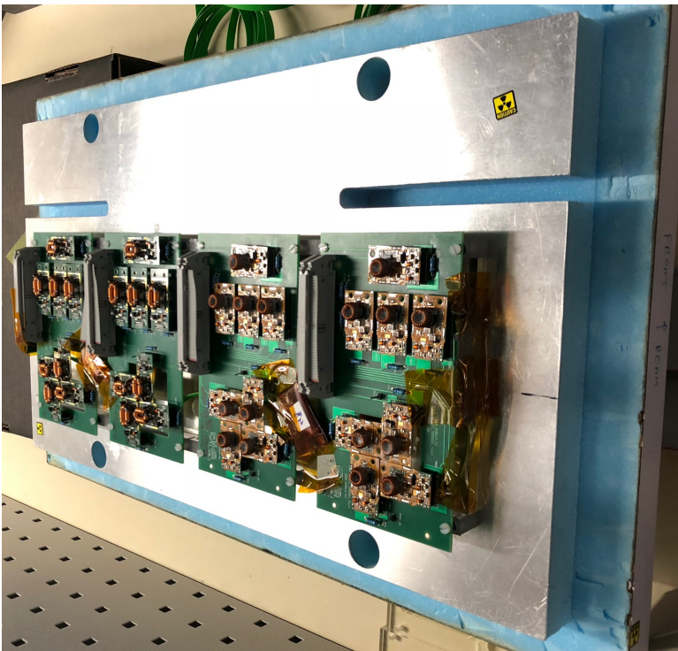
Figure 4: The 4 motherboards are installed on the cold box cover, ready for the exposure.
