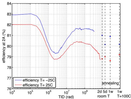
Figure 6: Efficiency variation with X-ray irradiation at the temperature of 25 and -25°C, for  $V_{in}=10V$ ,  $V_{out}=2.5V$  and  $I_{out}=2A$ . Measurements are taken immediately after each irradiation step (no annealing). The last TID point for 25°C is at about 700Mrad(SiO<sub>2</sub>).
