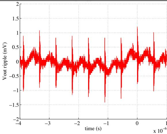
Figure 27: Output voltage ripple measured with an oscilloscope (AC coupled) with 20MHz bandwidth. Measurements conditions were  $V_{in}=10V$ ,  $V_{out}=2.5V$  and  $I_{out}=2A$ .
