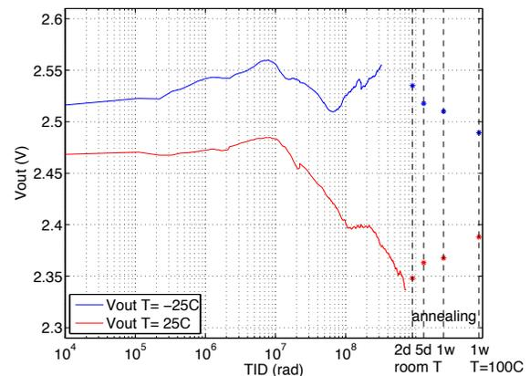
Figure 7: Output voltage variation with X-ray irradiation at 25 and -25°C, for  $V_{in}=10V$ ,  $V_{out}=2.5V$  and  $I_{out}=2A$ . Measurements are taken immediately after each irradiation step (no annealing). The last TID point for 25°C is at about 700Mrad(SiO<sub>2</sub>).
