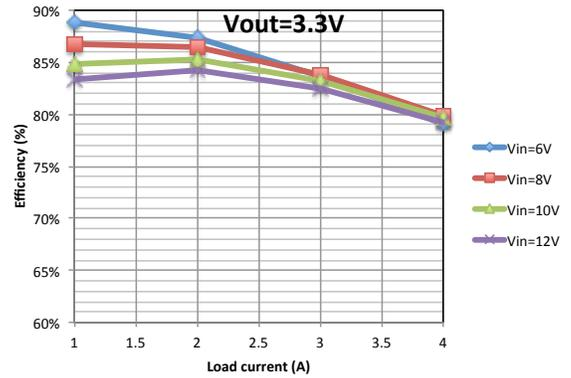
Figure 18: Efficiency for  $V_{out}=3.3V$  and different  $V_{in}$  and  $I_{load}$  with the module in good thermal contact with a cooling plate at about  $18^{\circ}C$ .
