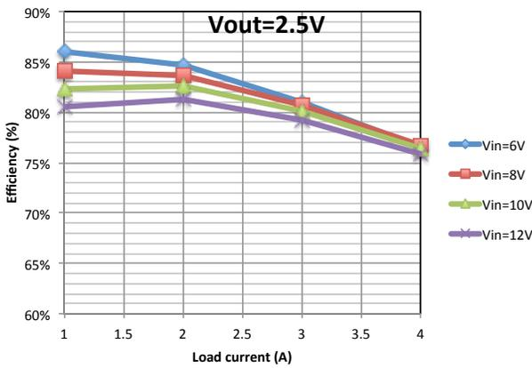
Figure 19: Efficiency for  $V_{out}=2.5V$  and different  $V_{in}$  and  $I_{load}$  with the module in good thermal contact with a cooling plate at about  $18^{\circ}C$ .
