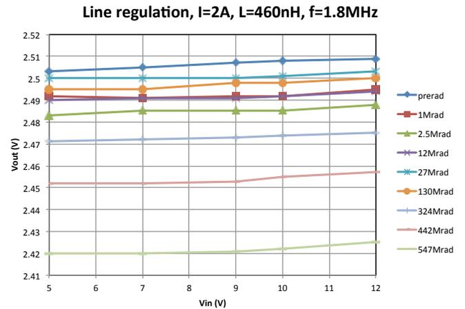
Figure 11: Line regulation variation with TID for an irradiation at 25°C. This module used the last ASIC prototype before the production-ready FEAST2.
