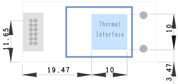
Figure 5: Top view of the module with size and position of the thermal interface.
