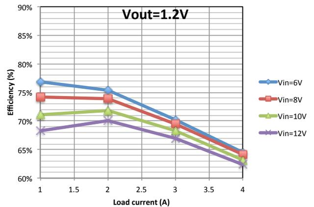
Figure 22: Efficiency for  $V_{out}=1.2V$  and different  $V_{in}$  and  $I_{load}$  with the module in good thermal contact with a cooling plate at about  $18^{\circ}C$ .
