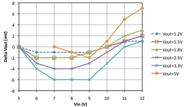
Figure 14: Line regulation for a load current of 4A with the module in good thermal contact with a cooling plate at about 18°C.
