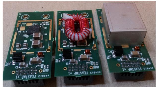
Figure 1: View of the FEASTMP module fully assembled (right), with shield removed (center) and with main inductor removed (left).
