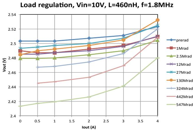
Figure 10: Load regulation variation with TID for an irradiation at 25°C. This refers to measurements taken on the module, before the output pi filter: the impact of the parasitic resistance of the filter's inductor and of the power connector is not included (but these do not change with TID). This module used the last ASIC prototype before the production-ready FEAST2.
