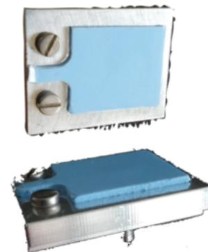
Figure 29: The pre-cut thermal pad, of a light blue color, is here positioned on top of a metal cooling plate fitting the FEASTMP module – the 2 screws fit the holes in the module and secure it to the metal plate that should be in contact with the cooling system.
