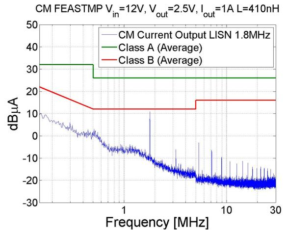
Figure 25: Output common mode current of the typical FEASTMP module at  $V_{in}=12V$ ,  $I_{out}=1A$ , and for  $V_{out}$  of 1.2V (left) and 2.5V (right). Noise is kept below the Class B limit of the CISPR11 reference standard, with only the fundamental at the switching frequency exceeding 0 dBµA. Lowering the input voltage leads to a sensible decrease of the noise currents.
