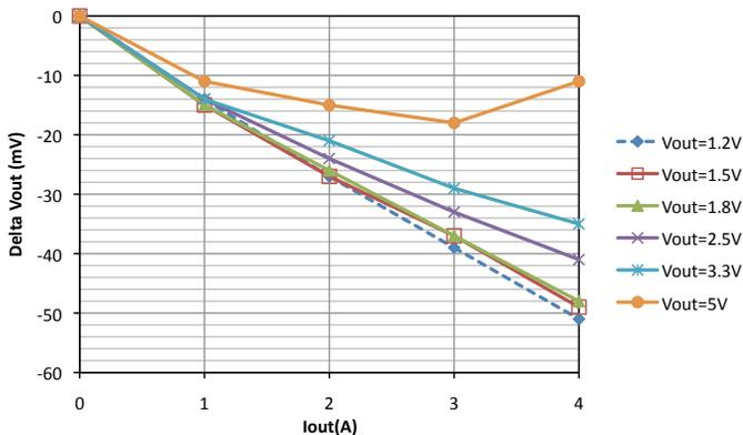
Figure 15: Load regulation for Vin=10V (very similar at all other input voltages). The drop is almost linear and it is due to the parasitic series resistance of the inductance of the output filter and of the power connector. At high output voltages, the linear decrease
