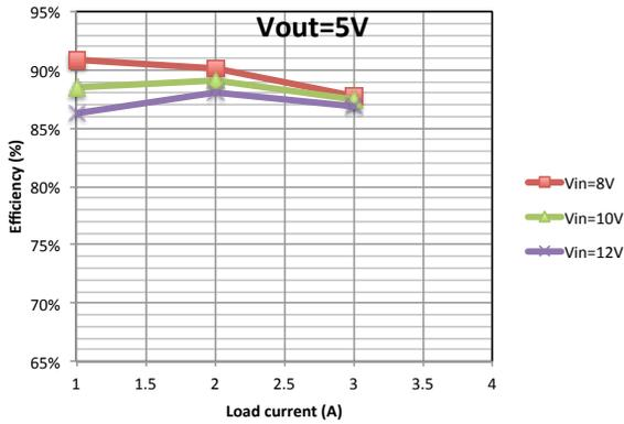
Figure 17: Efficiency for  $V_{out}=5V$  and different  $V_{in}$  and  $I_{load}$  with the module in good thermal contact with a cooling plate at about  $18^{\circ}C$ . The points at 3A are already beyond the max specified output power of 10W and are reported only for completeness.  $V_{in}$  needs to be at least 2V above  $V_{out}$ , therefore there is no curve for  $V_{in}=6V$ .
