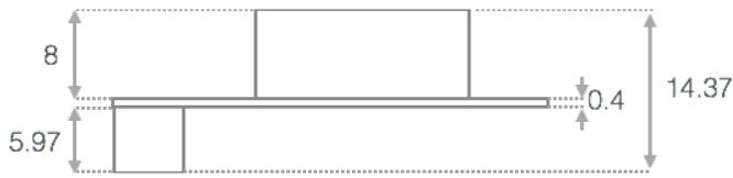
Figure 3: Side view of the FEASTMP module with mechanical dimensions.
