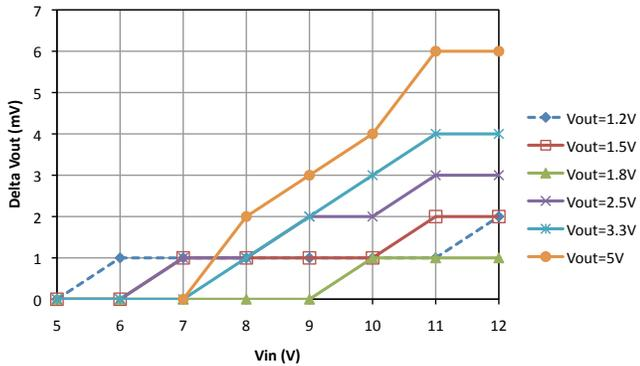
Figure 13: Line regulation for a load current of 2A with the module in good thermal contact with a cooling plate at about 18°C.
