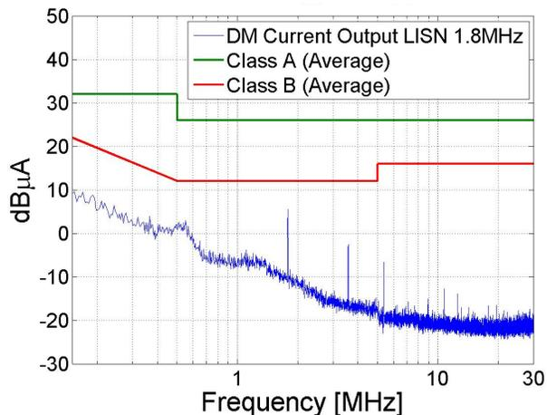
Figure 26: Output differential mode current of the typical FEASTMP module at  $V_{in}=12V$ ,  $I_{out}=1A$  and for  $V_{out}=2.5V$ . All
