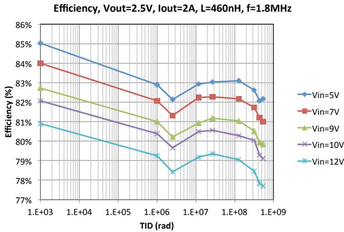
Figure 8: Efficiency variation with X-rays at 25°C, at different input voltages, and for 2A of load current (2.5V output). Last TID point is about 550Mrad(SiO<sub>2</sub>). This module used the last ASIC prototype before the production-ready FEAST2.
