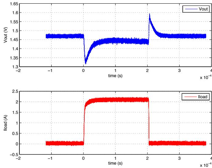
Figure 23: Transient load (0 to ~2A in ~5us) at  $V_{out}=1.5V$ .  $V_{in}=10V$ .
