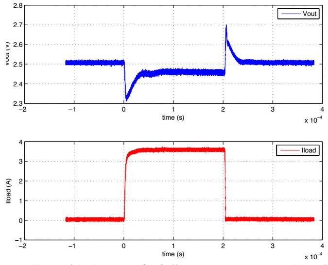
Figure 24: Transient load (0 to ~4A in ~5us) at  $V_{out}=2.5V$ .  $V_{in}=10V$ .
