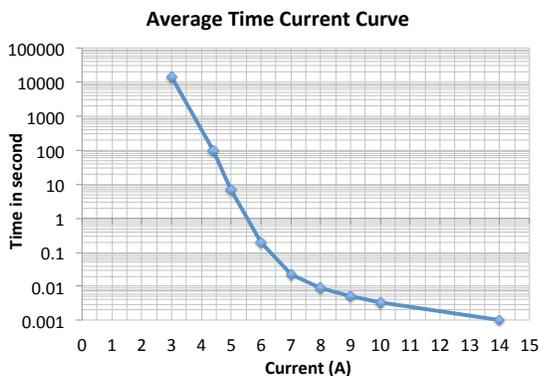
Figure 2: Average time for the fuse to burn and open the circuit.
