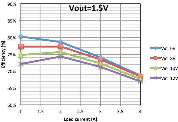
Figure 21: Efficiency for  $V_{out}=1.5V$  and different  $V_{in}$  and  $I_{load}$  with the module in good thermal contact with a cooling plate at about  $18^{\circ}C$ .
