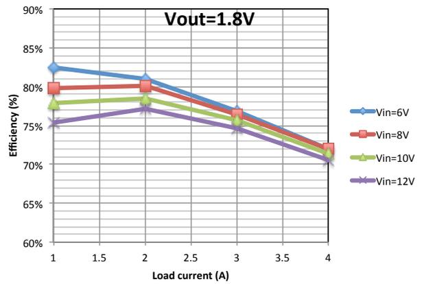
Figure 20: Efficiency for  $V_{out}=1.8V$  and different  $V_{in}$  and  $I_{load}$  with the module in good thermal contact with a cooling plate at about  $18^{\circ}C$ .
