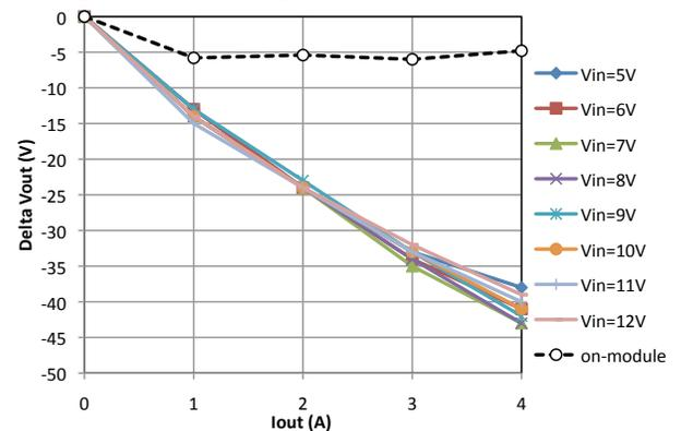
Figure 16: Load regulation for Vout=2.5V. The drop, independent on the input voltage, is almost linear and it is due to the parasitic series resistance of the inductance of the output filter and of the
