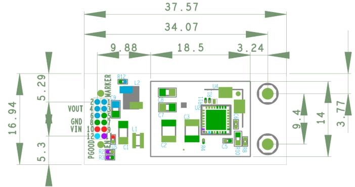
Figure 4: Top view of the FEASTMP module with mechanical dimensions.
