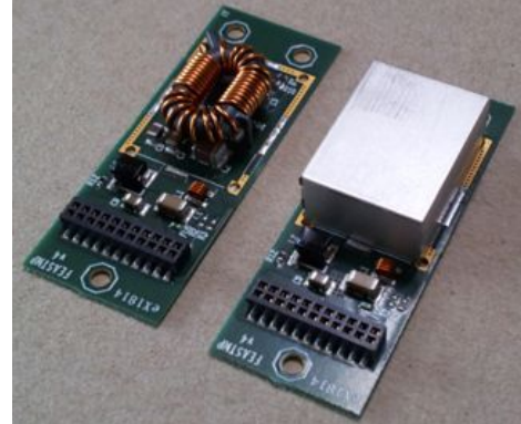
Figure 1: View of the FEASTMP_CLP module fully assembled (right) and with shield removed (left).
